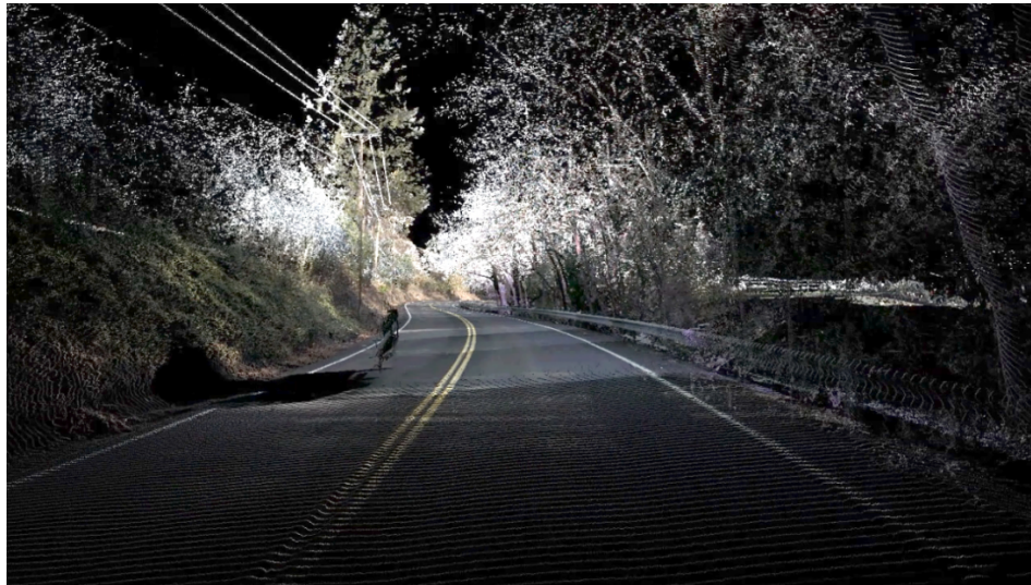
Figure 8: High Resolution 360 Degree View LiDAR Imaging (Public Domain)
