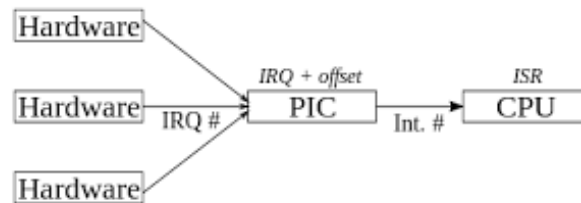
Figure 12: Hardware Interrupt Flow Diagram (Public Domain)
